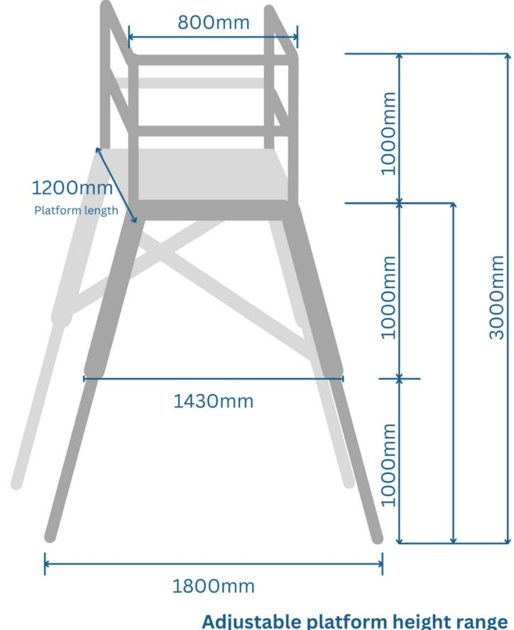
Adjustable platform height range Minimum - 1 metre Extended height - 2 metres
